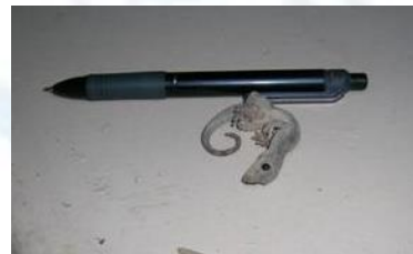
[Power outage accident caused by intrusion of a small animal]
