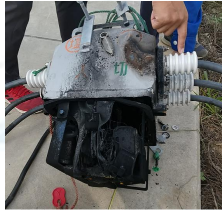
[Switchgear damaged by a lightning stroke]
